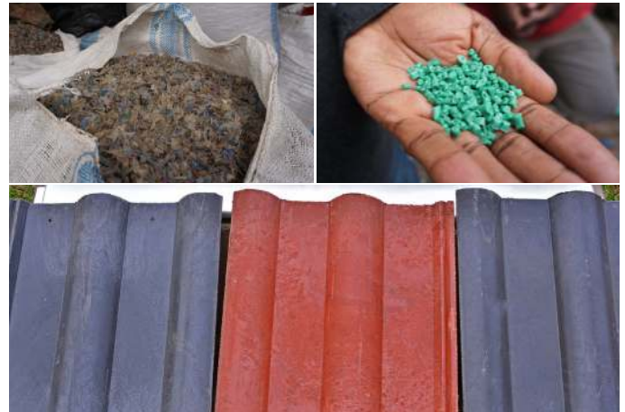
Plastic waste is crushed into small pieces and then turned into plastic flakes. Plastic flakes are used as raw material for plastic production. Final products from recycled plastic are for example roofing tiles by Ecoplastile Ltd.
